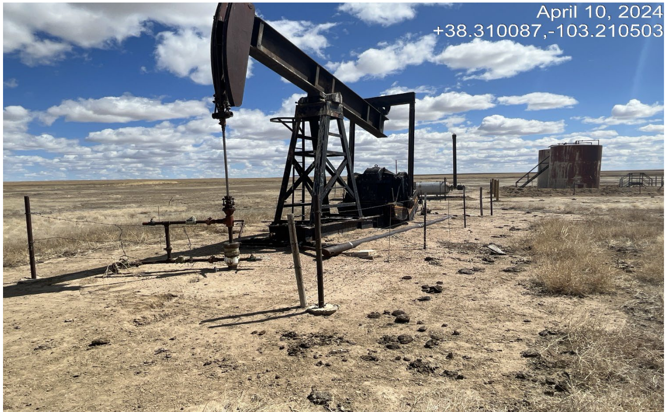
Photo 3. Facing toward the TA'd well. The pumpjack is not in use and needs to be removed.
