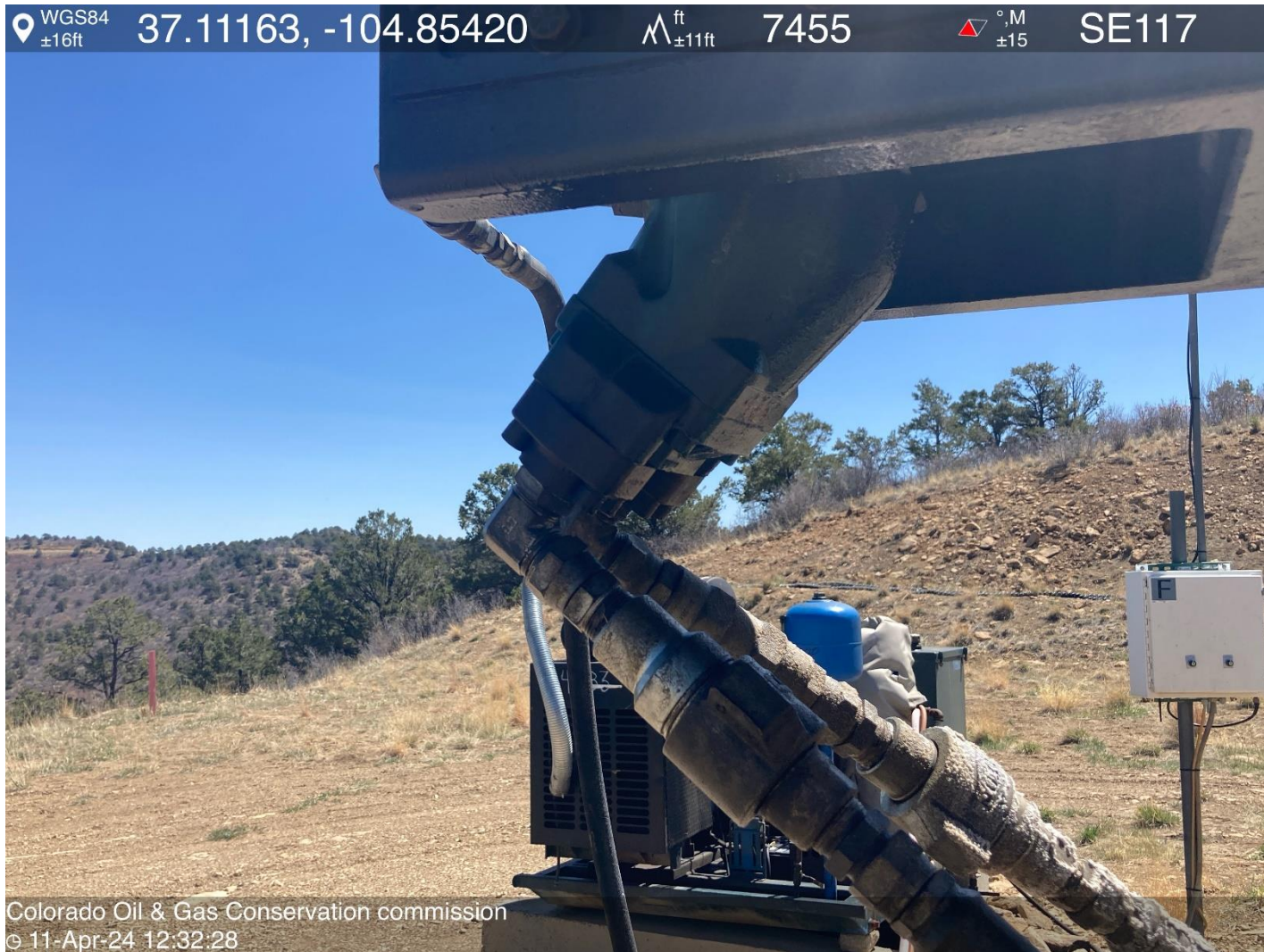
PHOTO 5: DRIVEHEAD IS LEAKING HYDRAULIC OIL (IT IS HARD TO SEE IN PHOTO HOWEVER THERE IS AN ACTIVE DRIP OF HYDRAULIC OIL DRIPPING OFF OF DRIVEHEAD NEAR HOSES ON GEAR BOX. Securely fasten all valves, pipes, fittings, and Production Facilities to ensure good mechanical condition, inspect at regular intervals and maintain in good mechanical condition per Rule 608.e. DUE TO ACTIVE LEAK REPAIR MUST BE DONE WITHIN 24 HOURS CA DATE 4-12-2024. LEFT A VOICMAIL FOR LAWRENCE BOWMAN REGARDING LEAKS.
