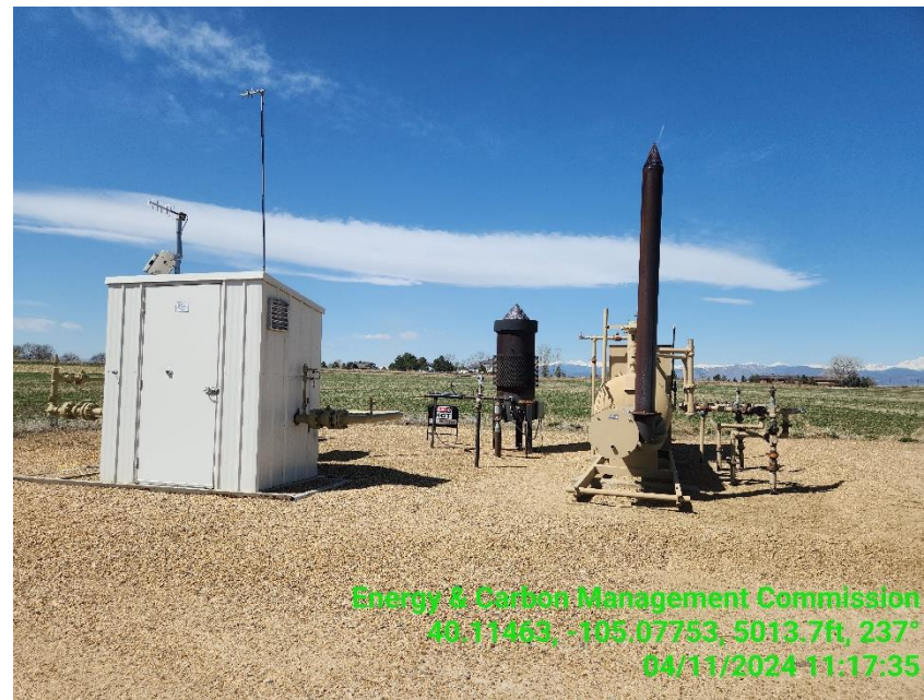
Photo 4 Gas Meter Run, card indicates current calibration. ECD & Horizontal Heated Separator.
