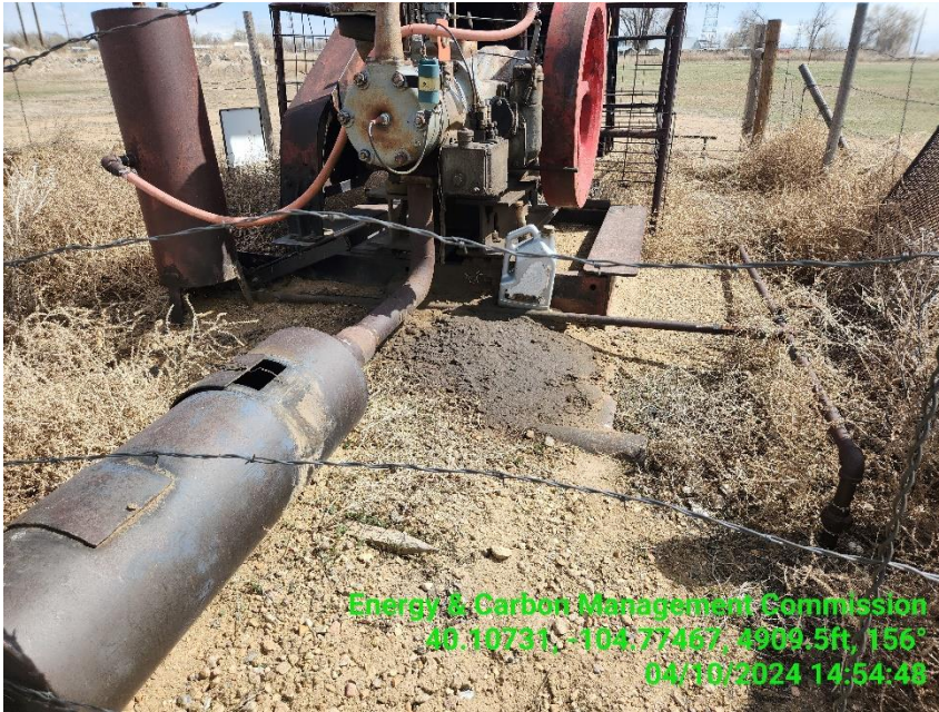
Photo 11 Dead vegetation/Stained soil by the prime mover (gas engine).
