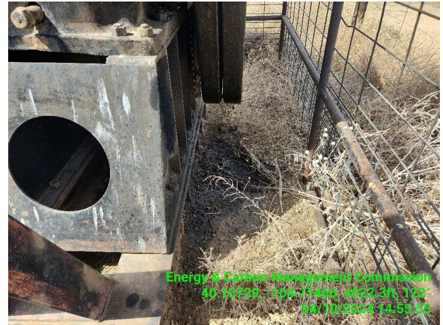
Photo 14 PJ base is over run with debris (dead vegetation) & the PJ gear box is leaking oil onto the ground.
