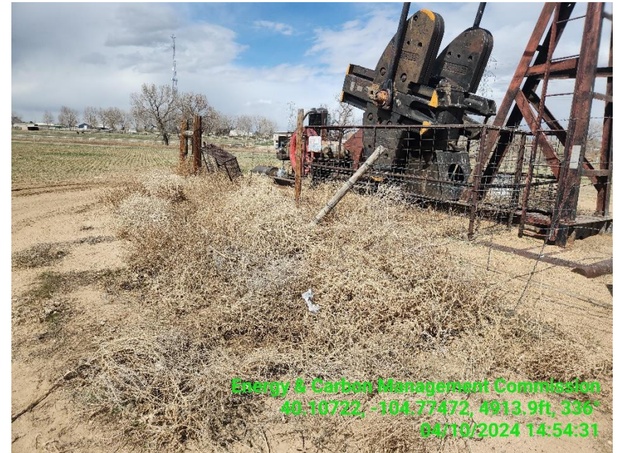
Photo 10 Pump jack base is over run with debris (dead vegetation)..
