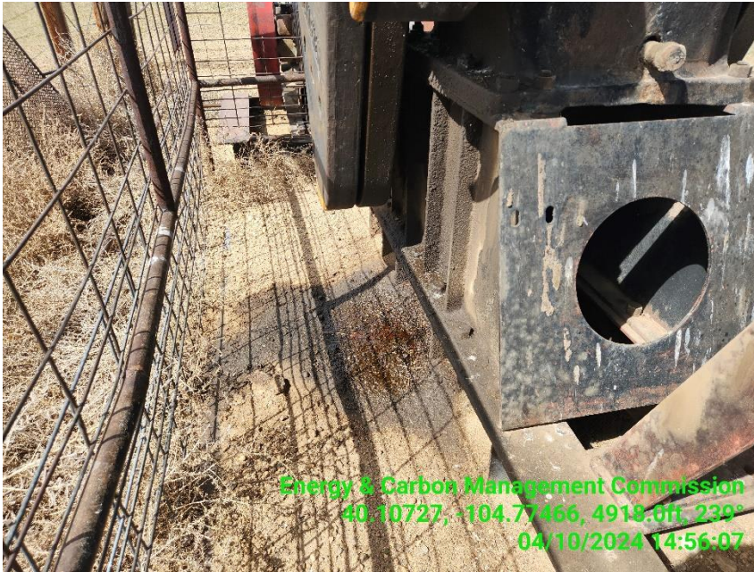
Photo 15 PJ gear box is leaking oil onto the ground.
