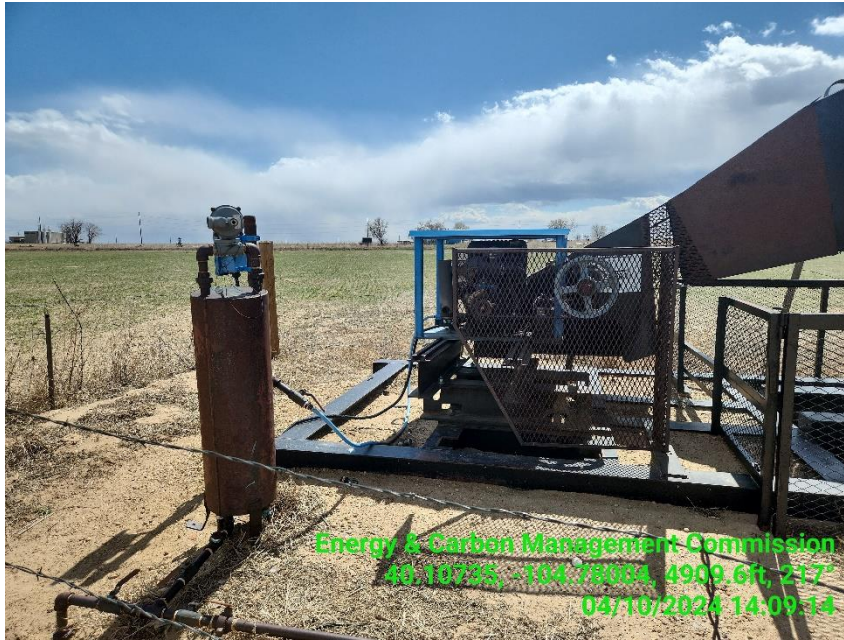
Photo 5 Prime mover (gas engine).
