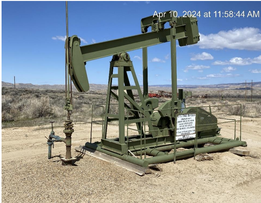
Pumping unit and wellhead
