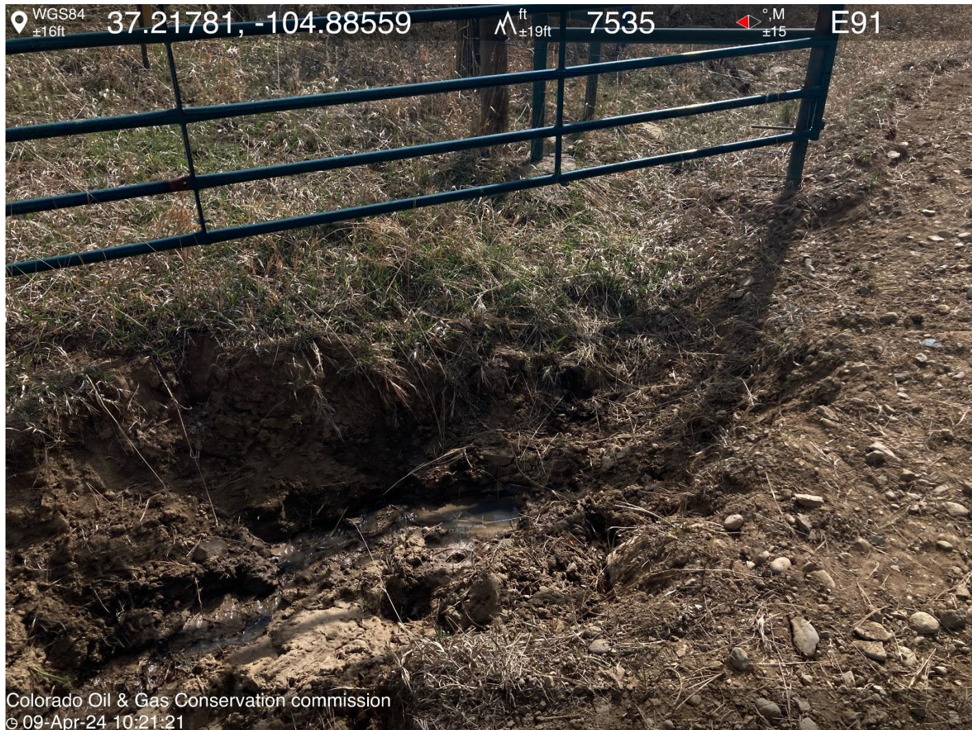
PHOTO 9: LEAK HAS ALMOST STOPPED AFTER PUMPER ISOLATED THIS GATHERING LINE.
