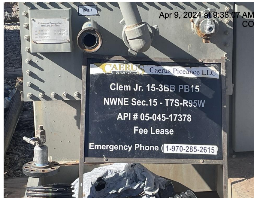
Photo # 3221 Open ended piping on separator/wildlife hazard/available for entry by wildlife
