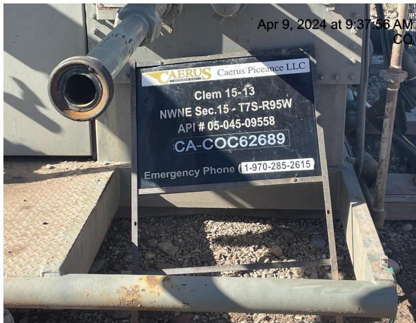
Photo # 3220 Open ended piping on separator/wildlife hazard/available for entry by wildlife
