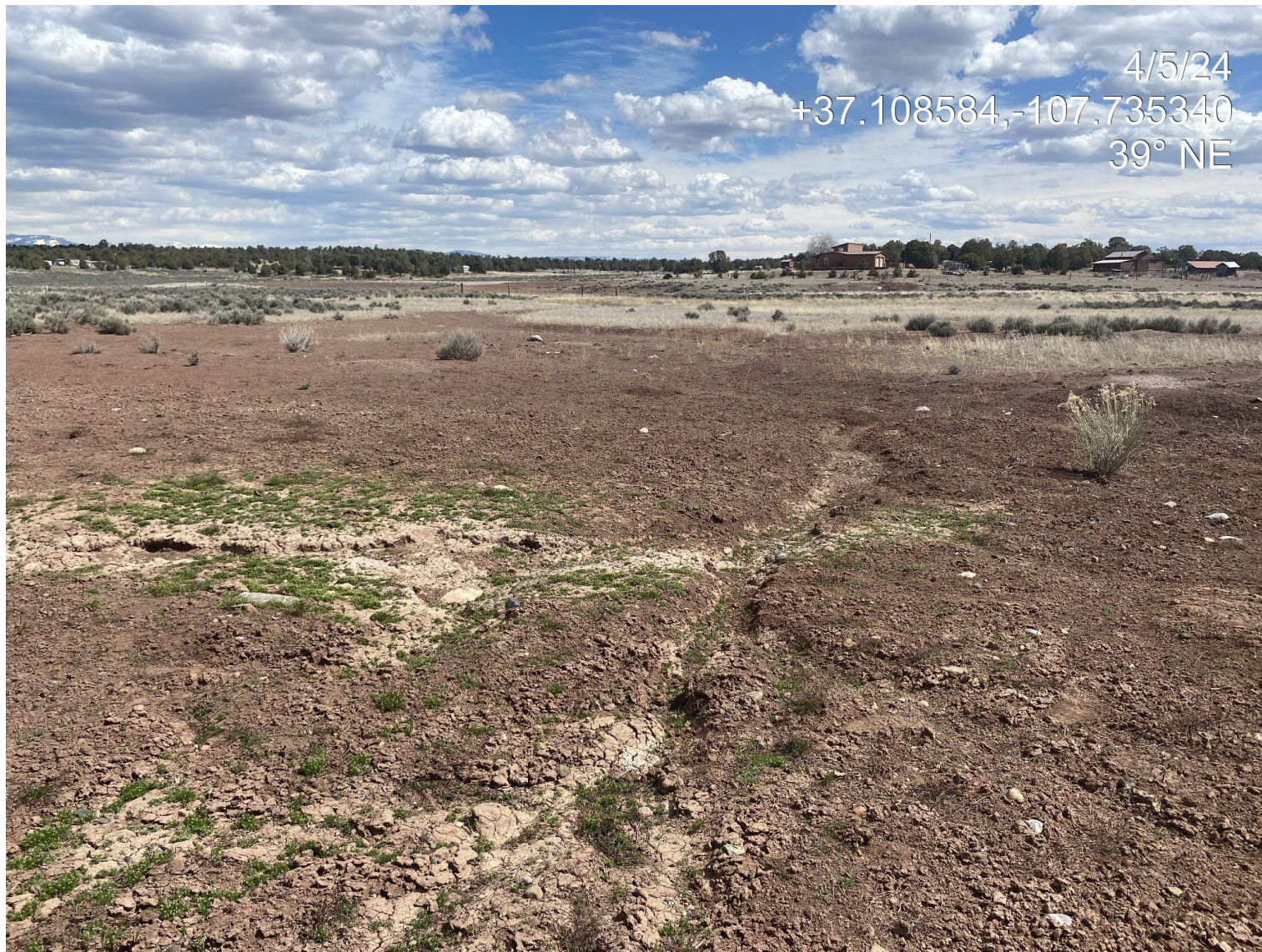
Photo 5. Rill erosion observed at the well head marker. Additional stabilization/storm water BMPs are needed in this area.
