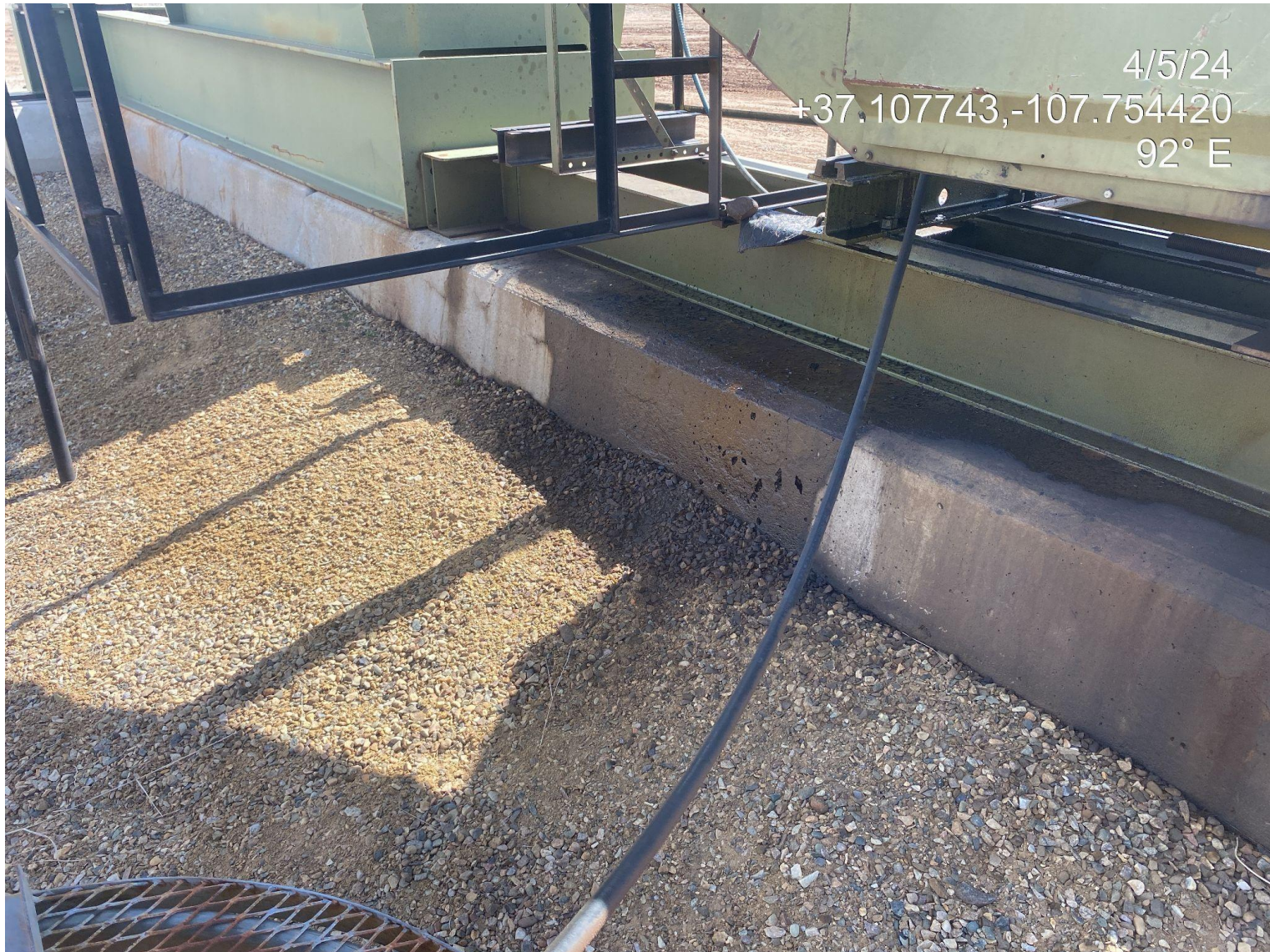
Photo 2. Stained surface material observed at Advanced Wireless Communications pump jack.
