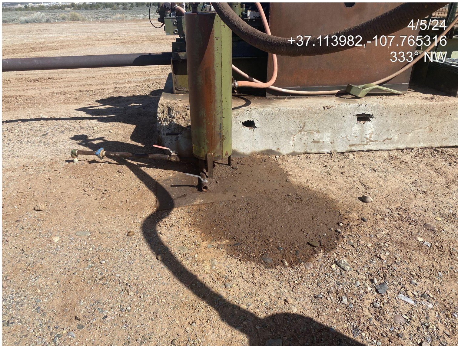
Photo 4. Impacted surface material observed at the mump jack muffler.
