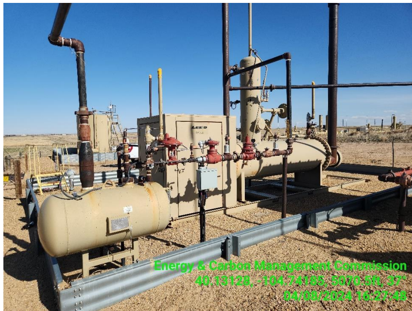
Photo 5 Horizontal Heated Separator.
