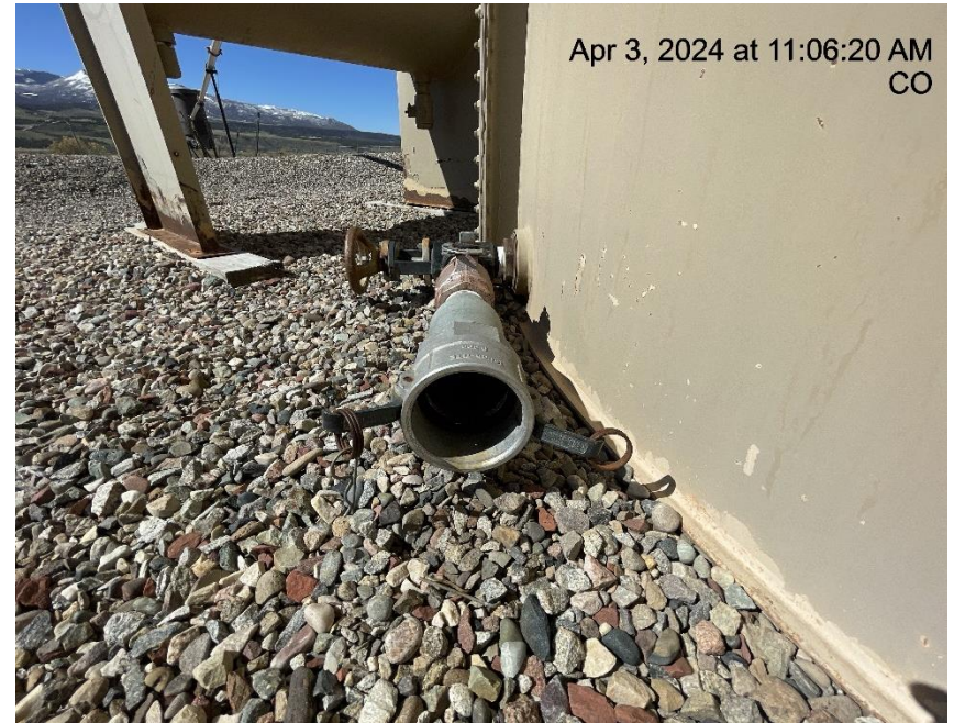
Photo # 2455 Open ended load line
