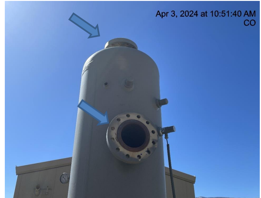
Photo # 2459 Openings on vessel available for entry by wildlife/wildlife hazards
