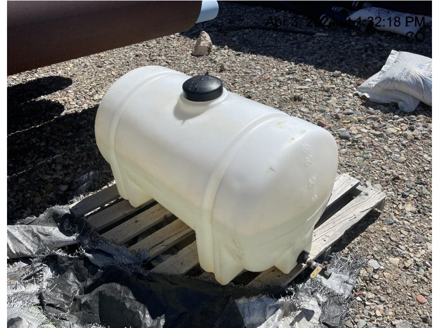
Photo # 2664 Chemical tank lacks containment/BMP (chemical tank is not labeled & is approximately half full of unknown fluid)
