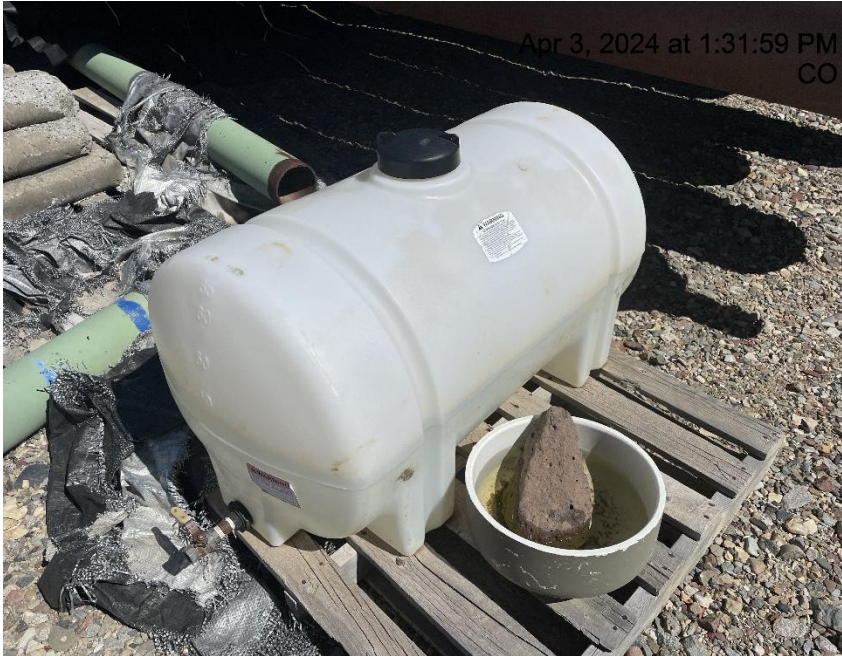
Photo # 2663 Chemical tank lacks containment/BMP (chemical tank is not labeled & is approximately half full of unknown fluid)
