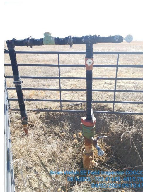
Wellhead with tubing valve closed
