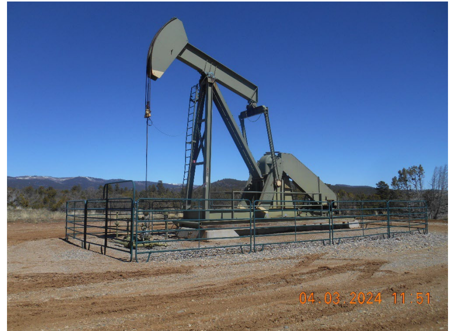
Wellhead with pump jack STATE #36-5 API #:05-067-08400
