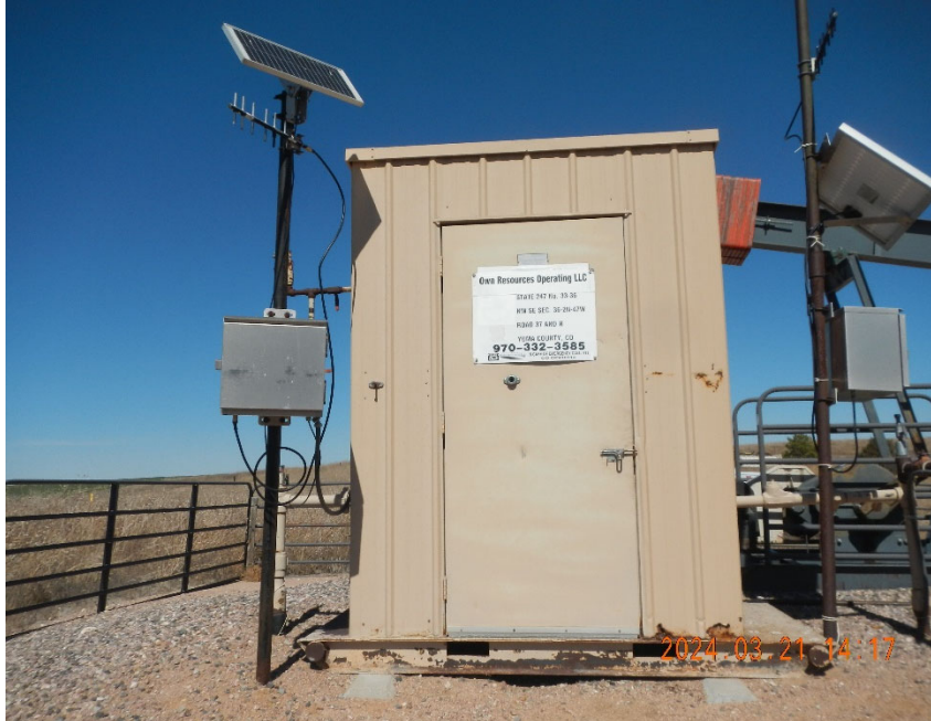
5. Remote Separator/meter shed for the State 247 33-36 well API# 125-07796 located on State 2-36-247 well pad.
