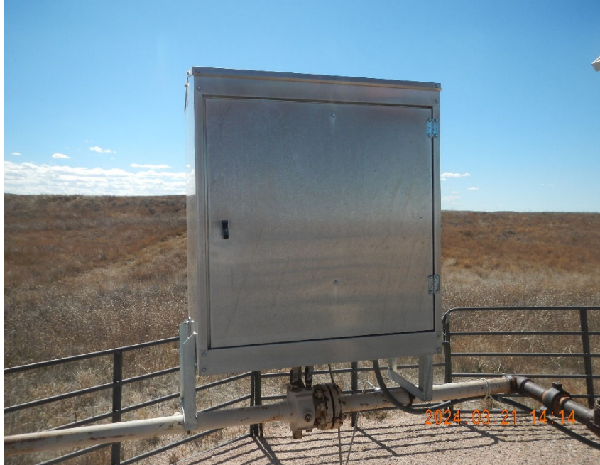
3. Flowline mounted meter box.
