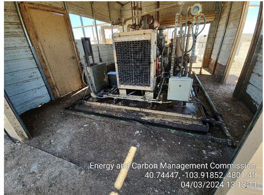
Photo 6 – Stained Soil at Compressor
