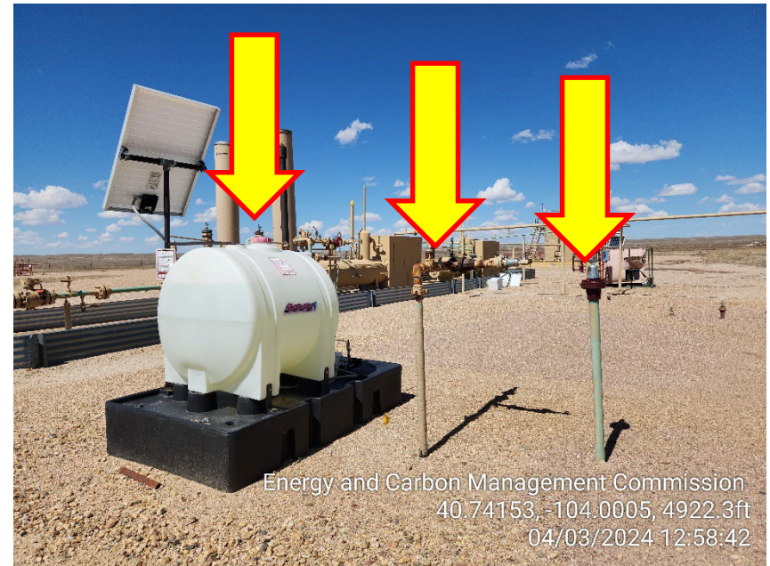
Photo 8 – Unused Chemical Contain at Compressor Site and Unmarked Risers
