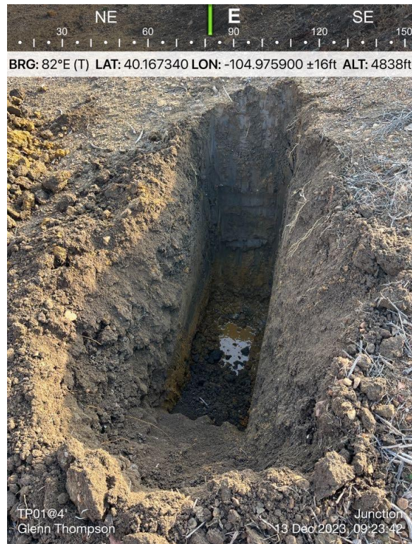
Groundwater in Test Pit 01 Excavation
