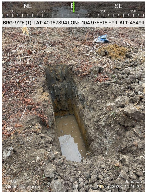
Ground Water in Test Pit 06 Excavation
