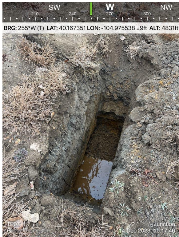
Ground Water in Test Pit 07 Excavation
