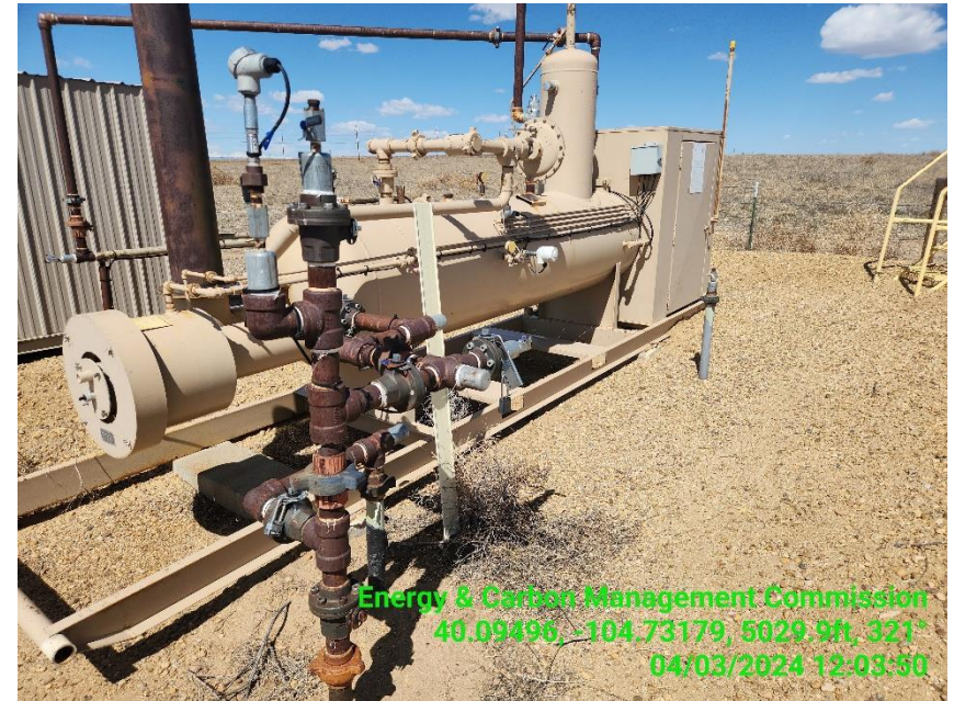
Photo 6 Horizontal Heated Separator is SI/LOTO.
