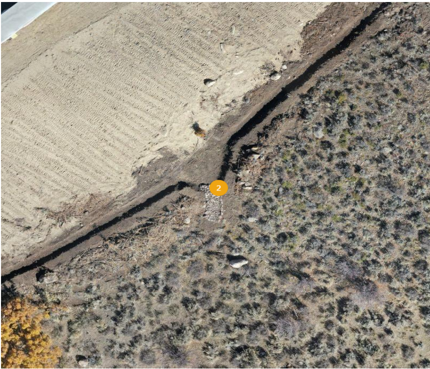
Details Operator has utilized topsoil material in the construction of the sediment trap BMP. This does not comport with Rule 1002.b. and 1002.c.
