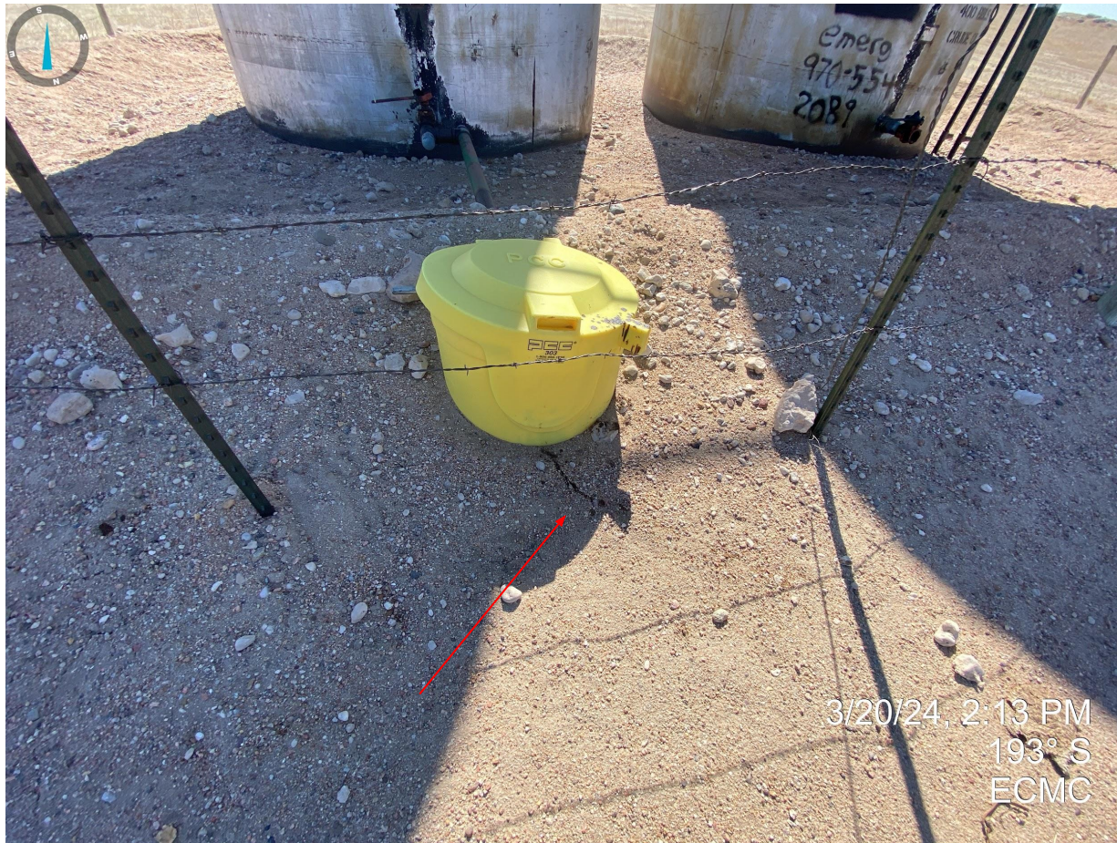
Photo 1. Stained soil observed at tank battery loadout line.
