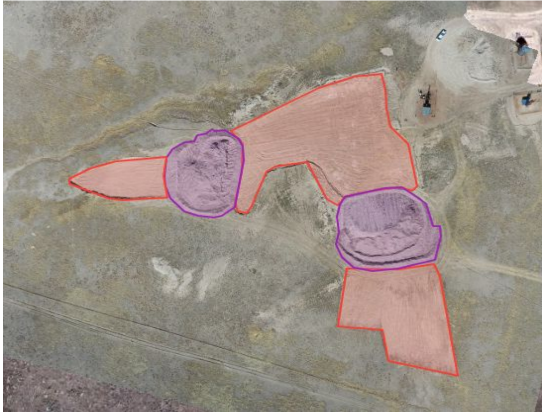
Photo 29. Drone aerial imagery captured 03/20/2024. Red shaded outlines illustrate (approx. 1.5 acres) of excavation within the former pit and salt kill areas. Purple shaded outlines (approx 0.75 acres, combined) indicate the soil stockpiles which are approximately 6300 CY in total (2700 CY for west stockpile and 3600 CY for east/south stockpile).
