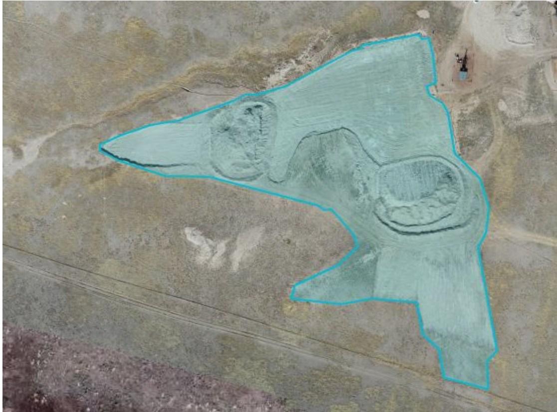
Photo 30. Drone aerial imagery captured 03/20/2024. Blue shaded outline illustrates a disturbance area of approximately 3.10 acres (excavation, stockpiles and salt kill impacted areas).
