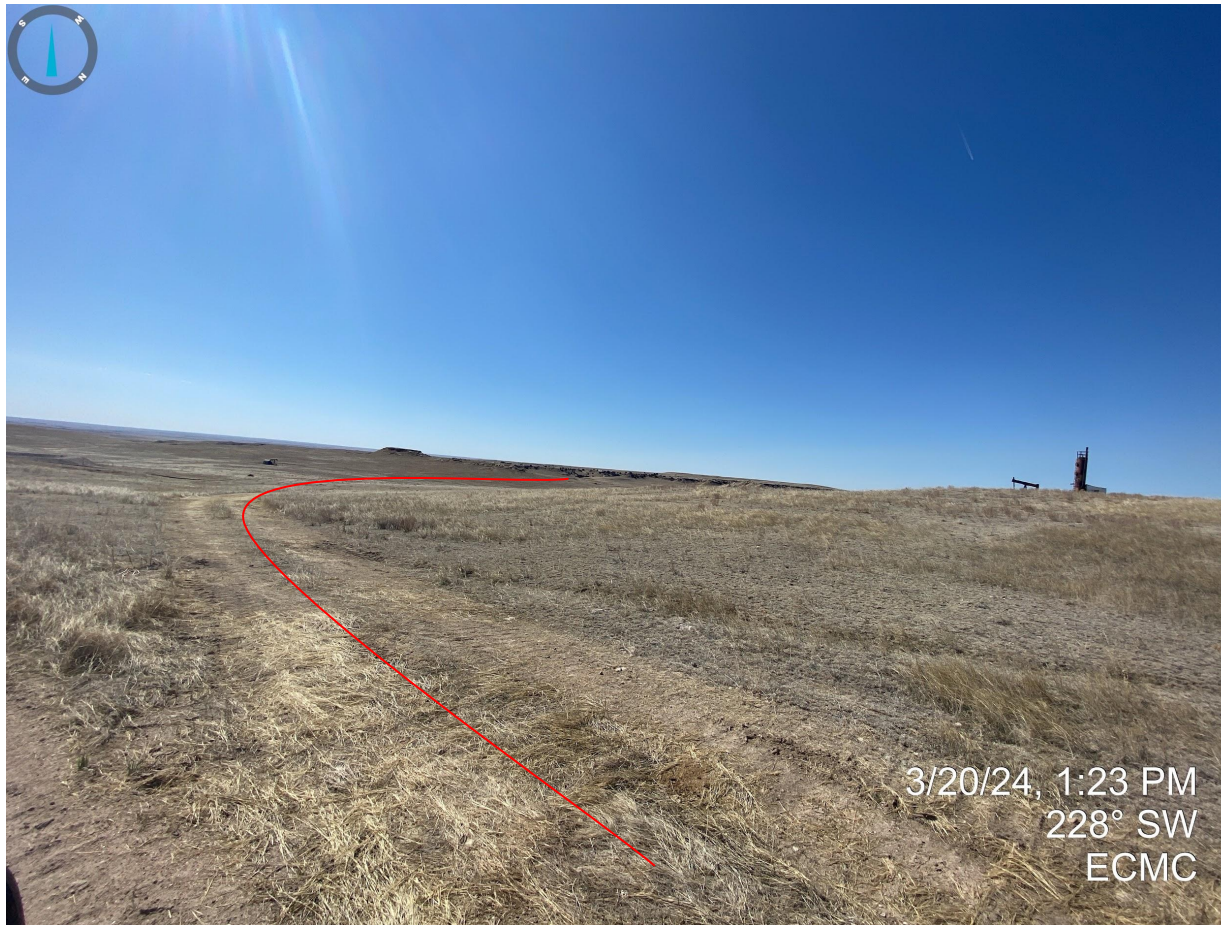
Photo 28. Taken east of the location along adjacent access road, illustrating traffic disturbance occurring outside of the permitted access roads. Red line illustrates vehicle traffic and associated disturbance that will need to be reclaimed per the reclamation rules.
