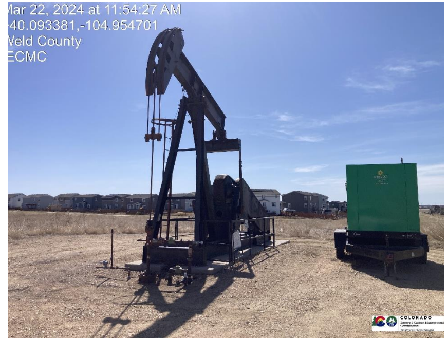
Pic 2 Wellhead / pump jack
