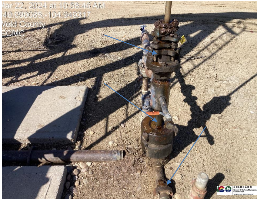
Pic 3 small leak on wellhead / contaminated soil
