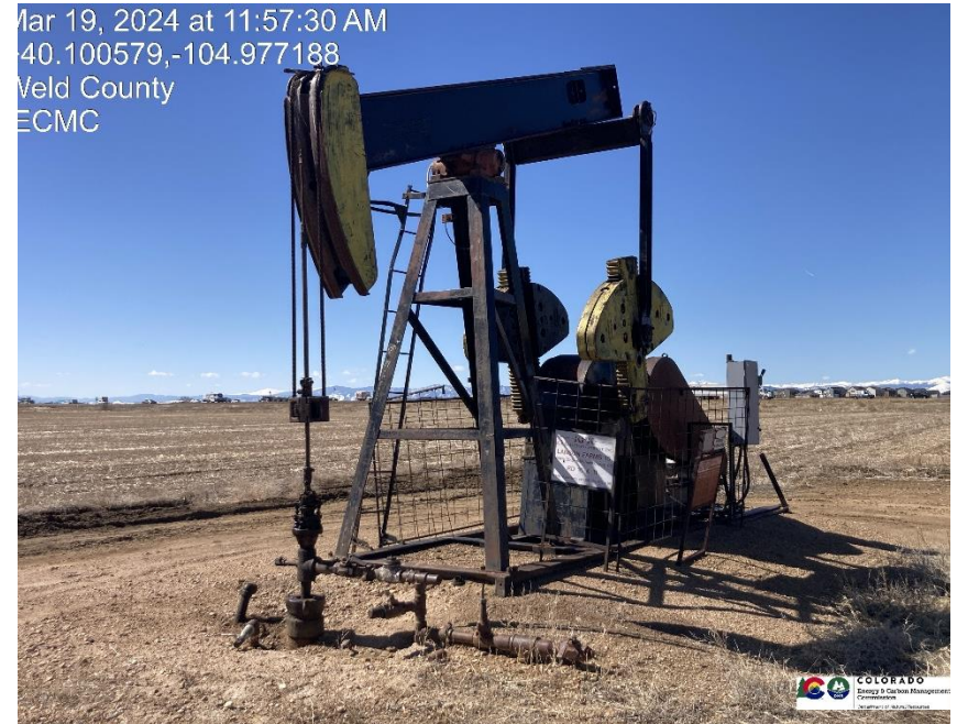
Pic 2 wellhead / pumpjack
