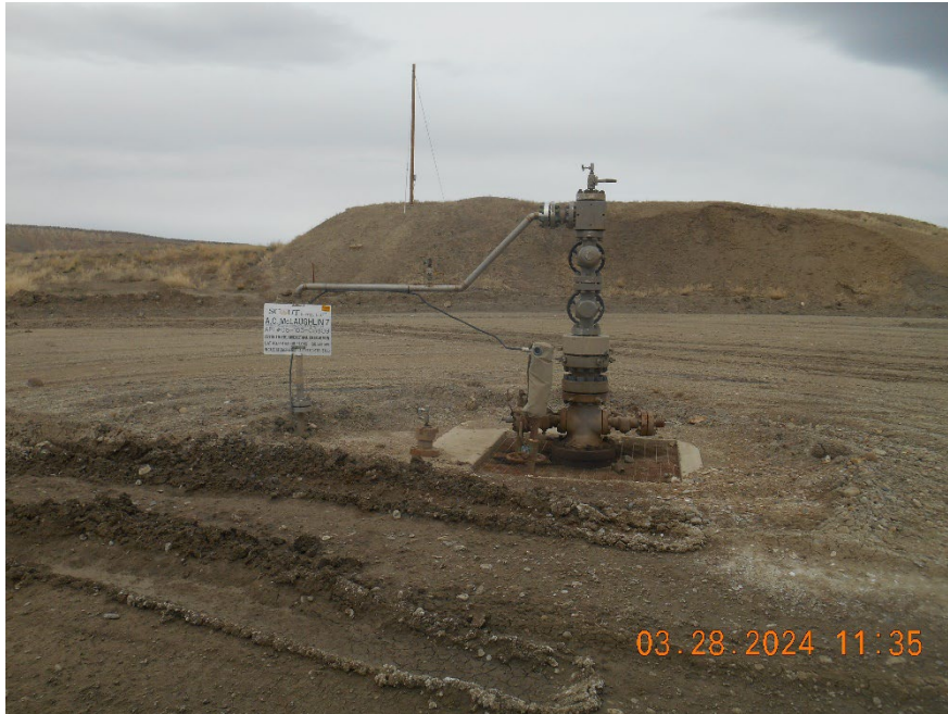
Injection Wellhead
