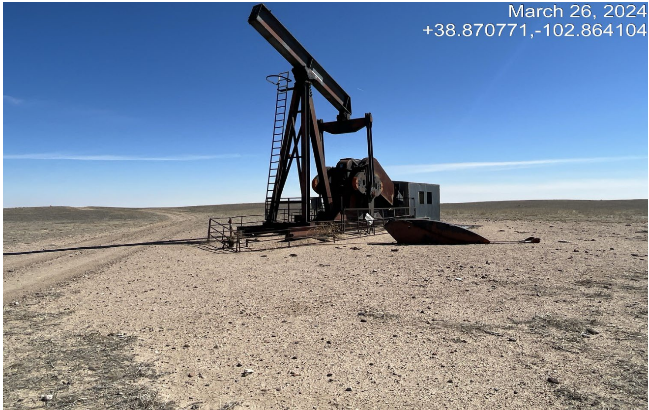
Photo 1. Facing northeast toward the wellsite. This well has been TA for a long time and all unused equipment needs to be removed.
