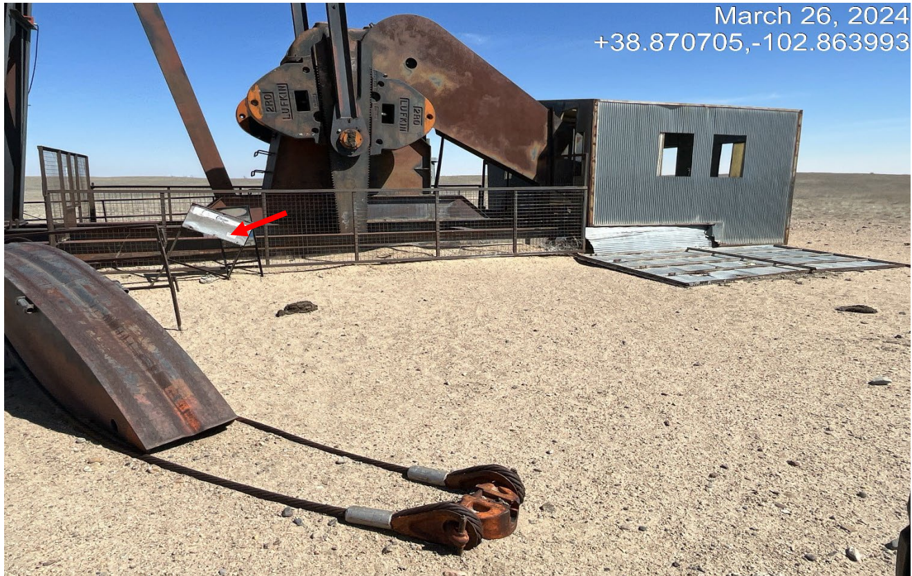
Photo 2. The well sign is faded and not legible. There is a metal panel pumpjack head laying on the ground.
