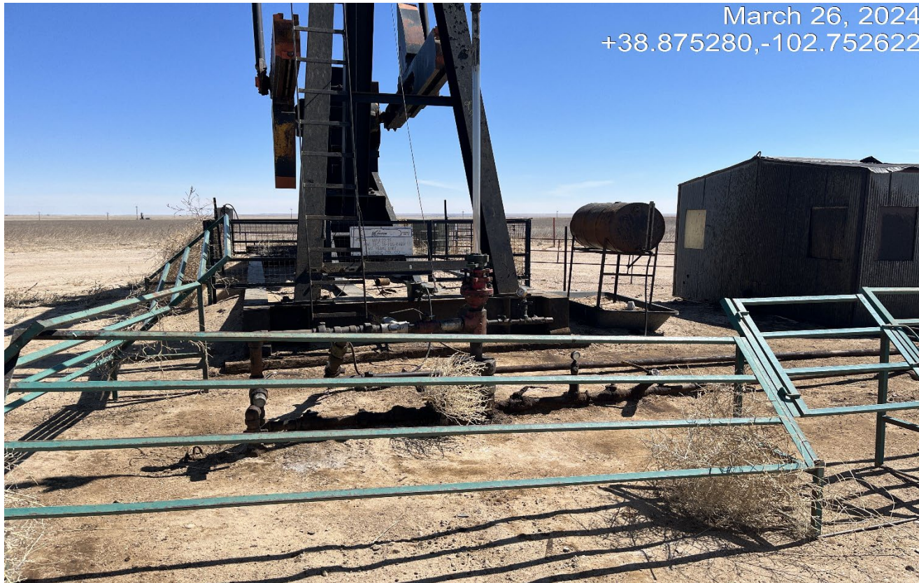
Photo 3. Facing toward the well. There are stained soils around the well which appear to have sprayed out oil to the south of the well.
