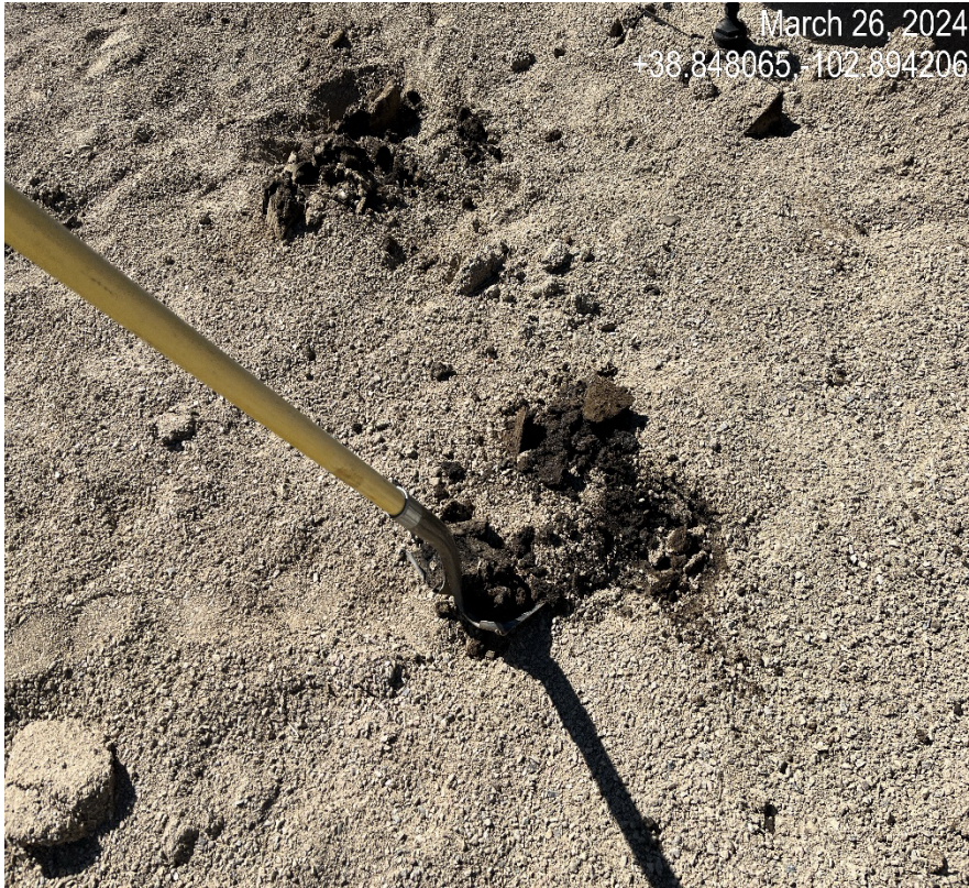
Photo 6. There is still oily soils and it appears material was spread over the spill to cover it up.
