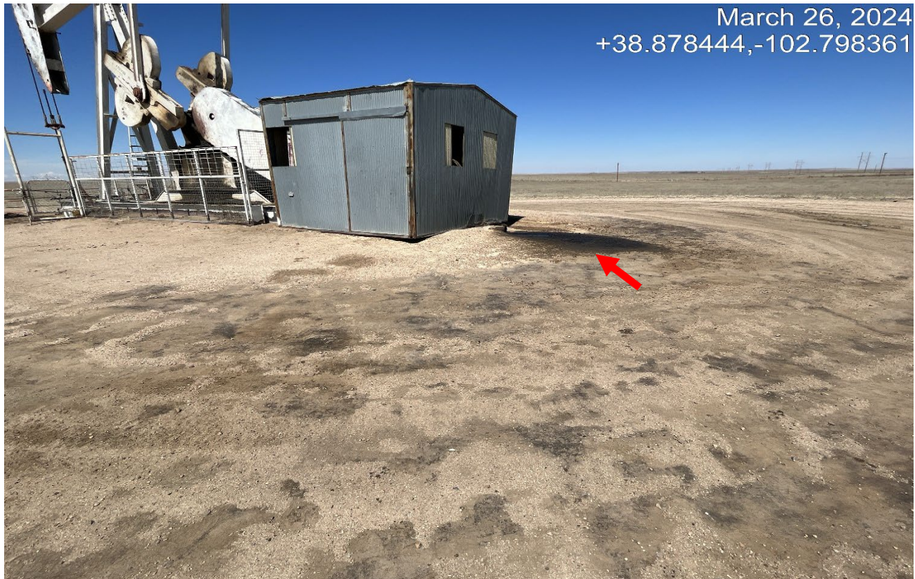
Photo 7. There is oil coming out of the exhaust pipe which is staining the soil and needs to be cleaned up.
