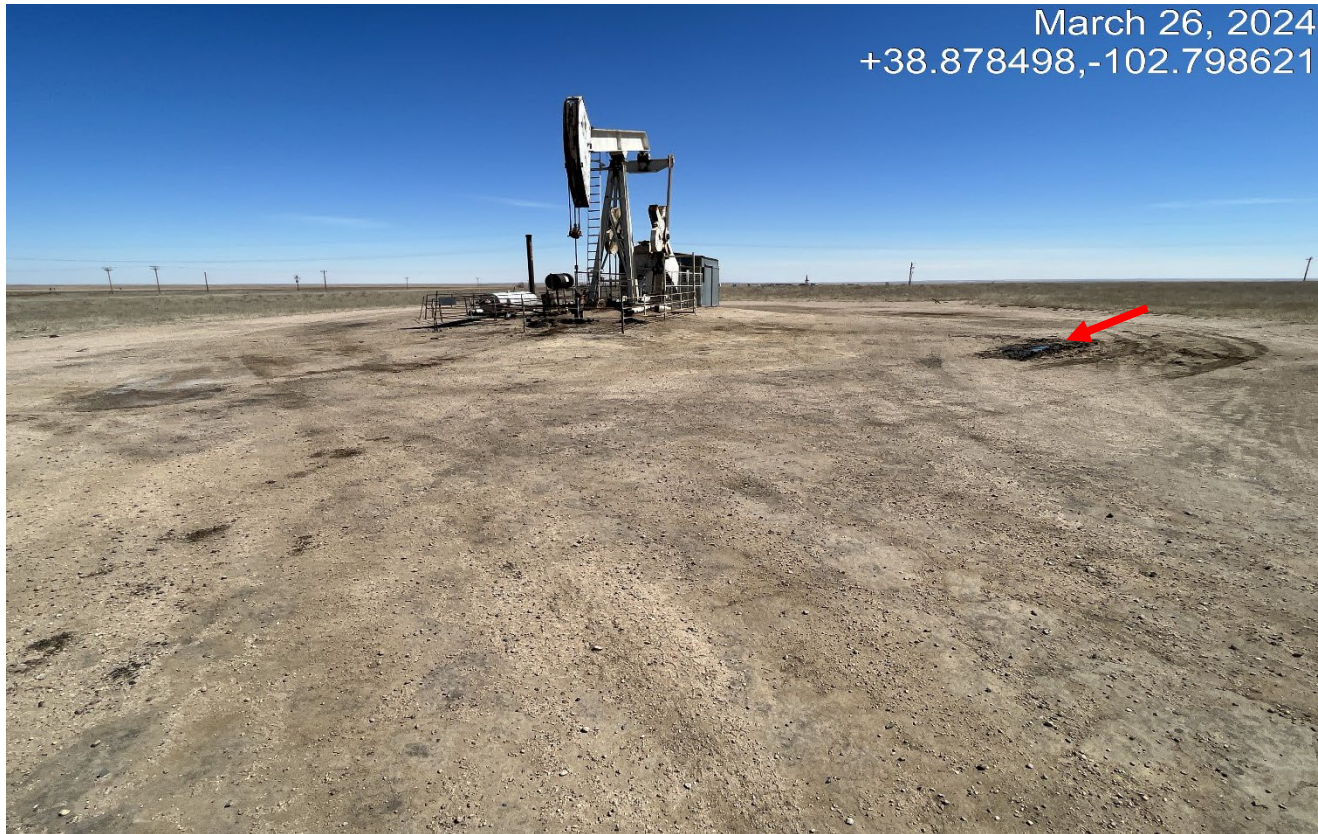
Photo 2. Facing east at the wellsite. There is oily waste pooled up on the surface shown at red arrow.
