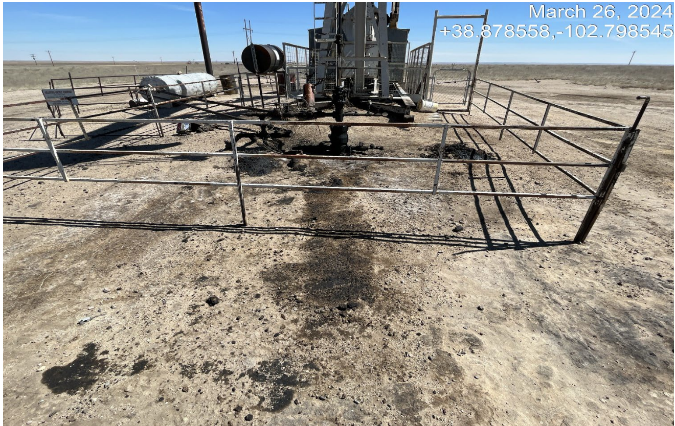
Photo 5. There is a spill that occurred at the wellhead with an undetermined amount spilled which will require a spill report.
