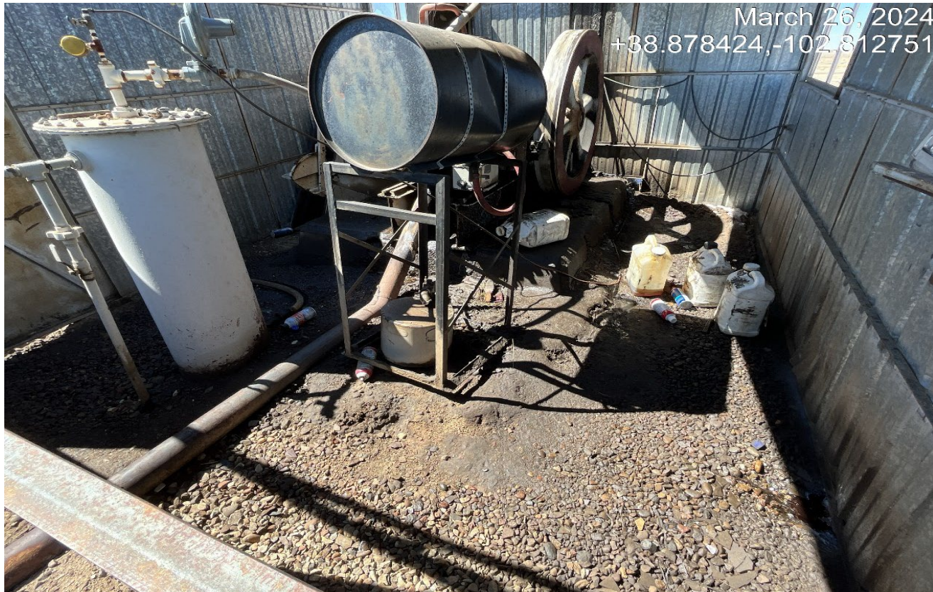
Photo 5. View of inside the shed shows oil saturated soils from the leaking engine. There is oil containers tipped over and no secondary containment.
