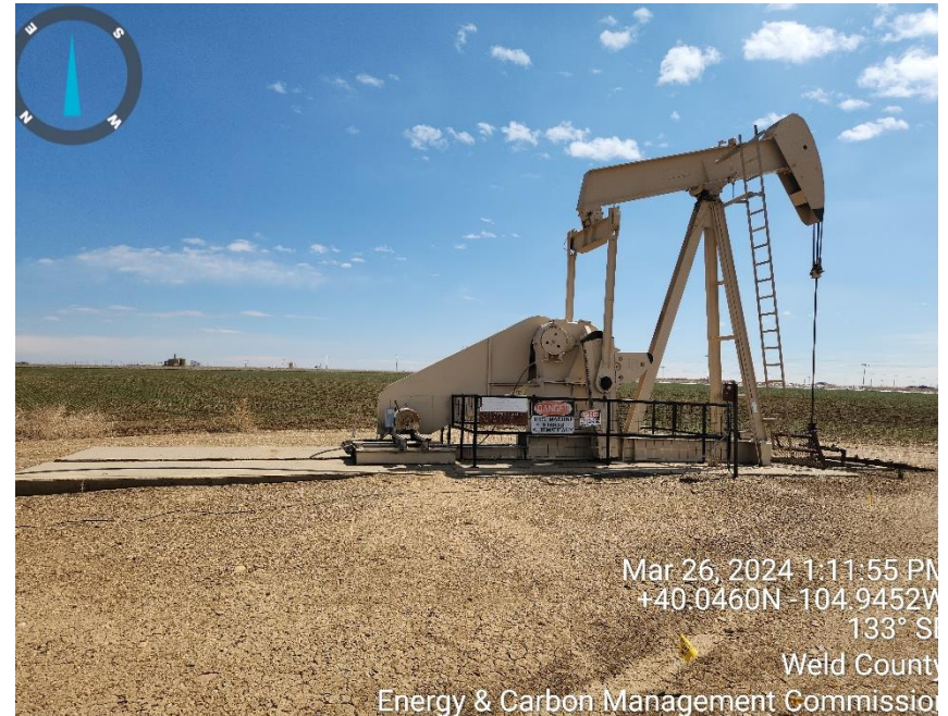
Photo 2 well head and equipment
