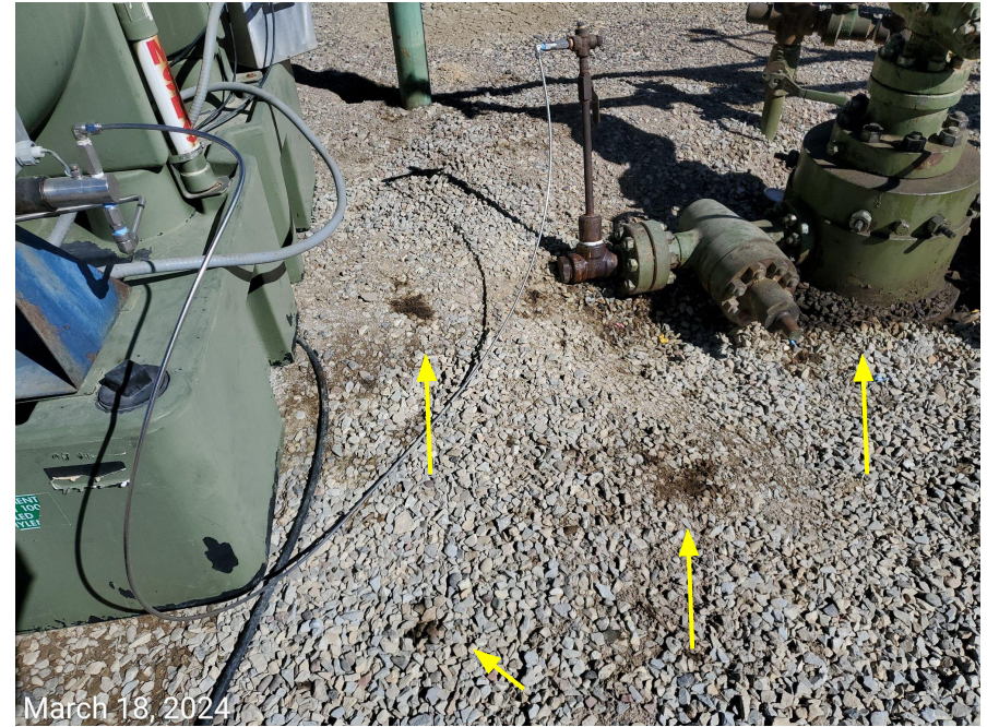
Photo 8: Photos show stained soils at the B-19N-N3 well (API 103-10836)
