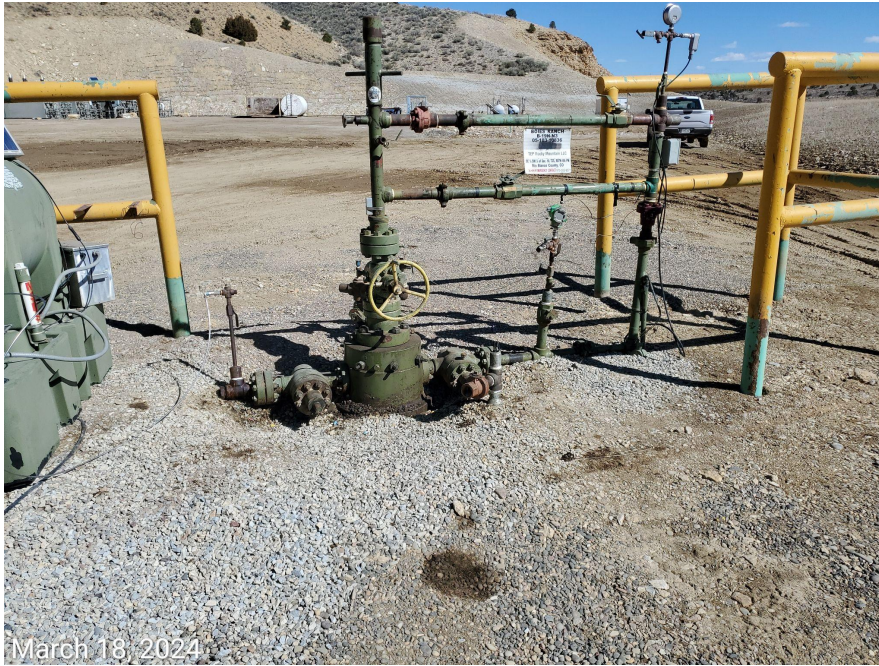
Photo 8: Photos show stained soils at the B-19N-N3 well (API 103-10836)
