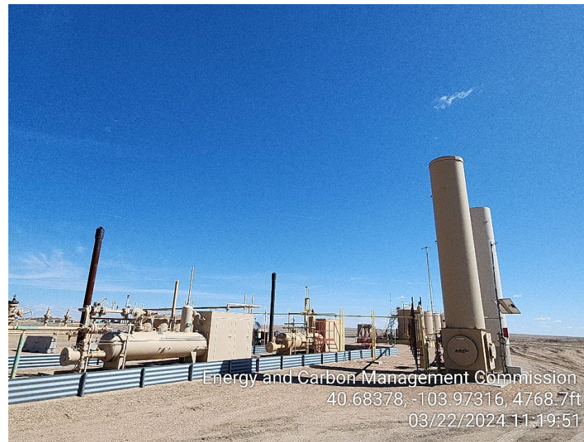
Photo 2 – ECDs and Separators
