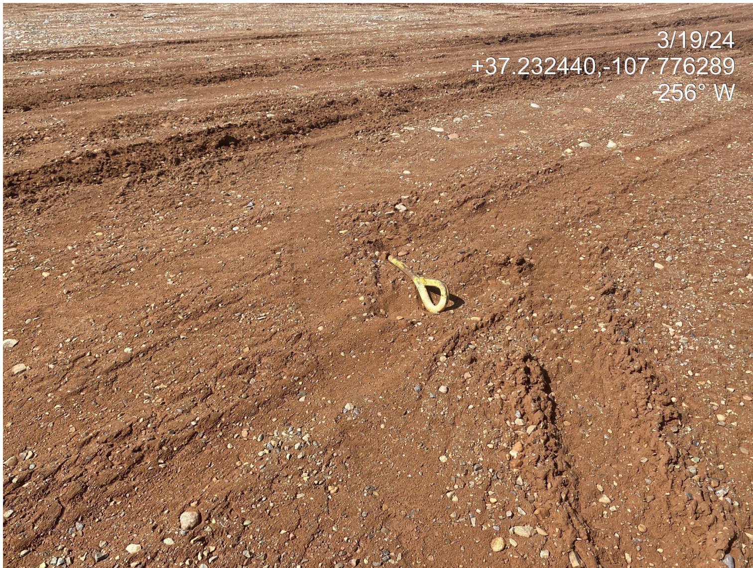
Photo 5. View of unmarked guy line anchor on location.
