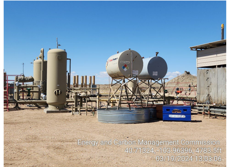
Photo 20 – Day Tanks at Compressor
