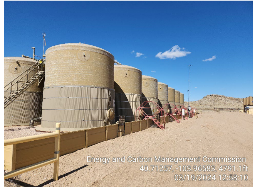
Photo 2 – Produced Water Tanks
