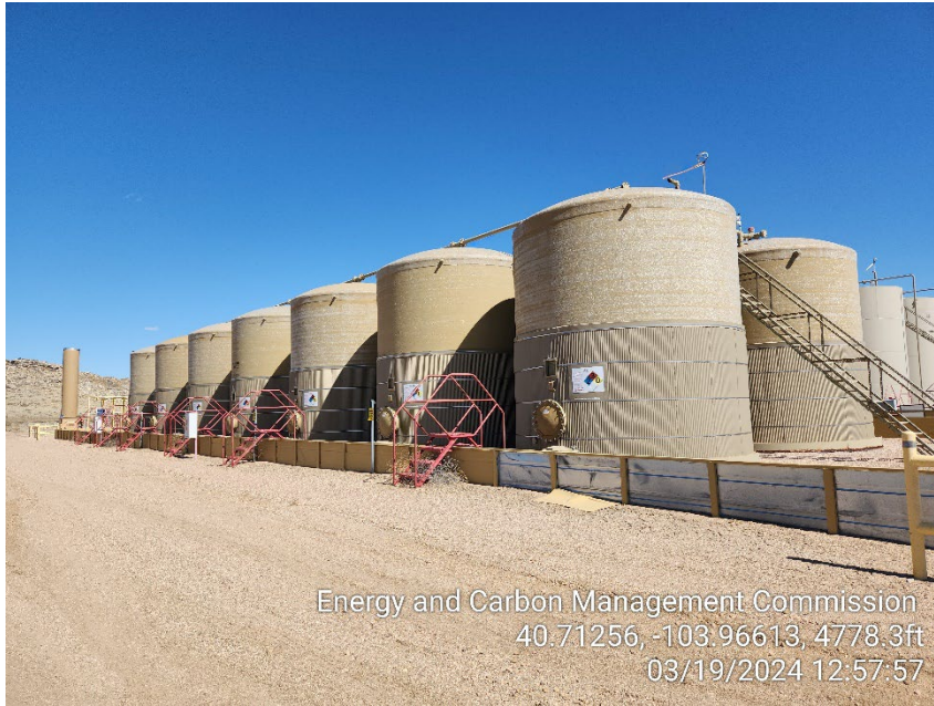
Photo 1 – Produced Water Tanks
