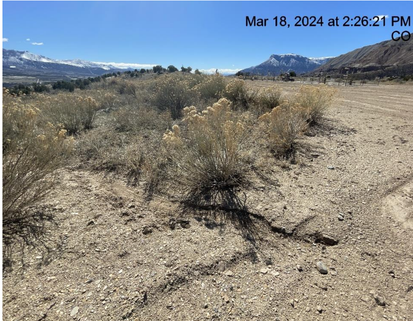
Photo # 323 Erosion & transport of sediment off location & into a vegetated area
