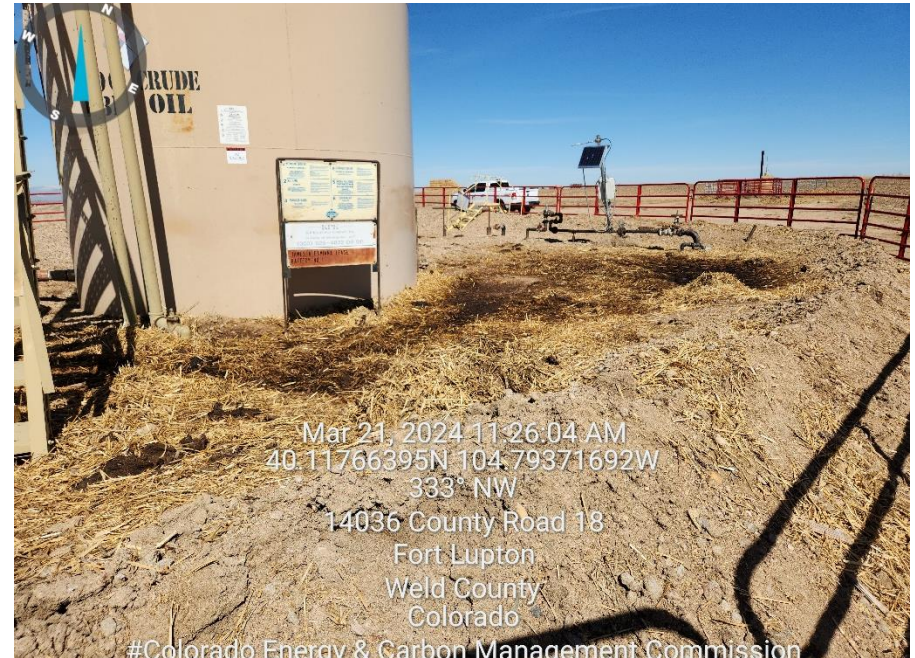
Photo 2 TNK BTRY sign rusted and not legible
