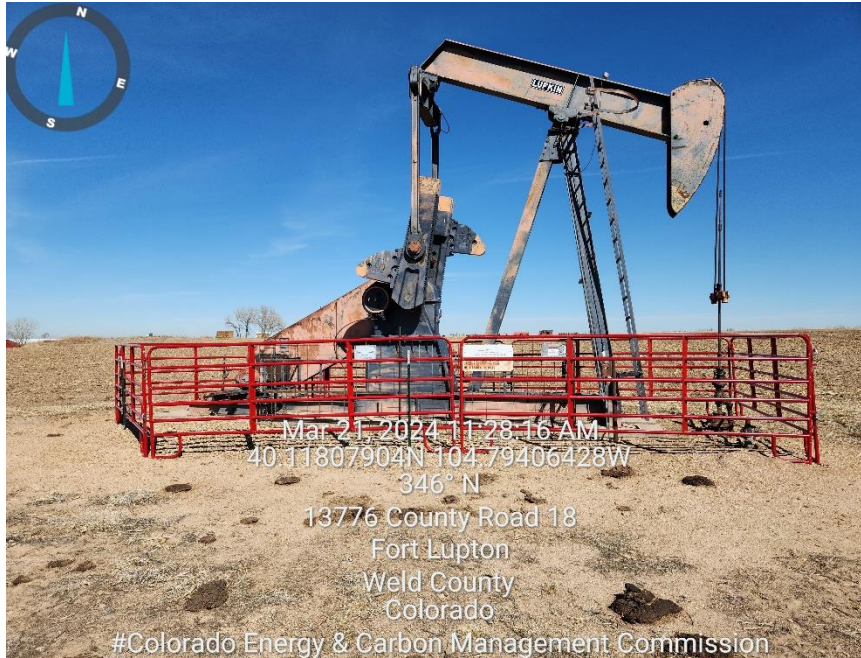
Photo 7 Well head sign faded not legible
