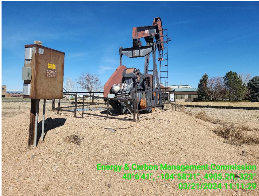
Photo 7 Electric panel, electric motor & pump jack.
