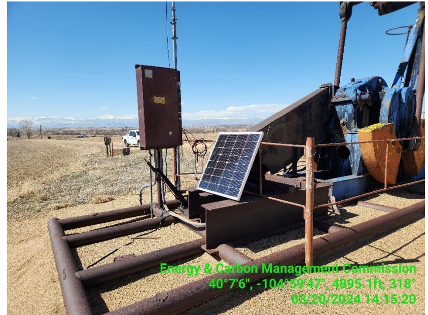
Photo 6 electric panel/monitoring equipment.
