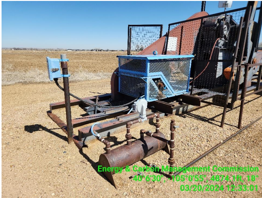
Photo 5 Prime mover (gas engine).
