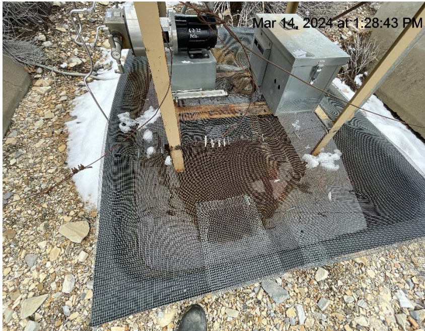
Photo # 182 Failure to maintain chemical BMP/Chemical containment approximately 1/2 to 5/8 full of fluid/BMP insufficient to contain possible spill.
