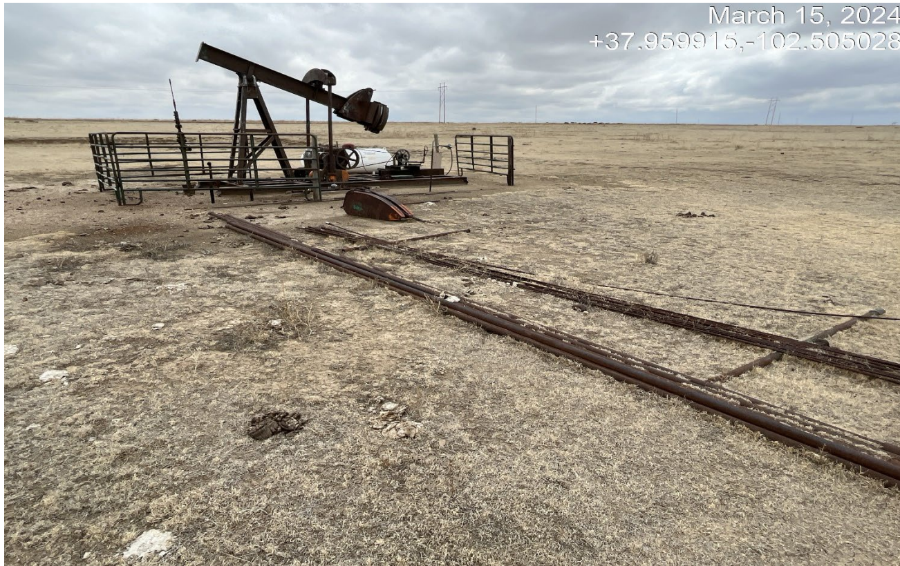
Photo 4. Facing toward the well. There is unused equipment and drilling pipe that needs to be removed..
