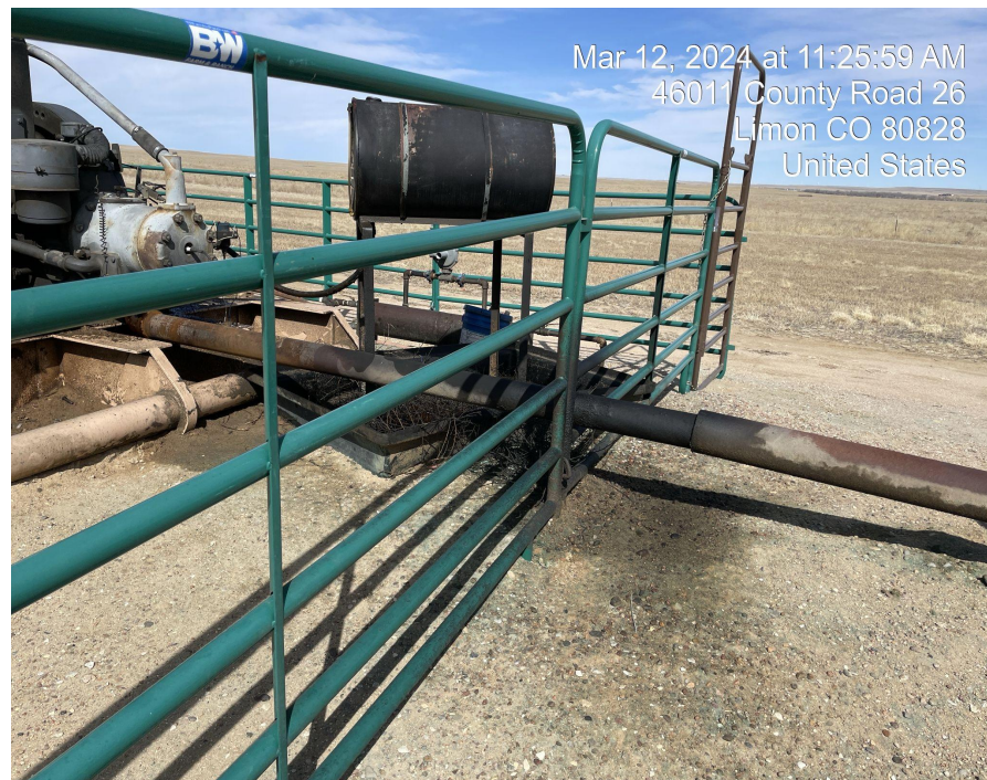
Photo 6. Photo taken facing north of stained soil around secondary containment and equipment.
