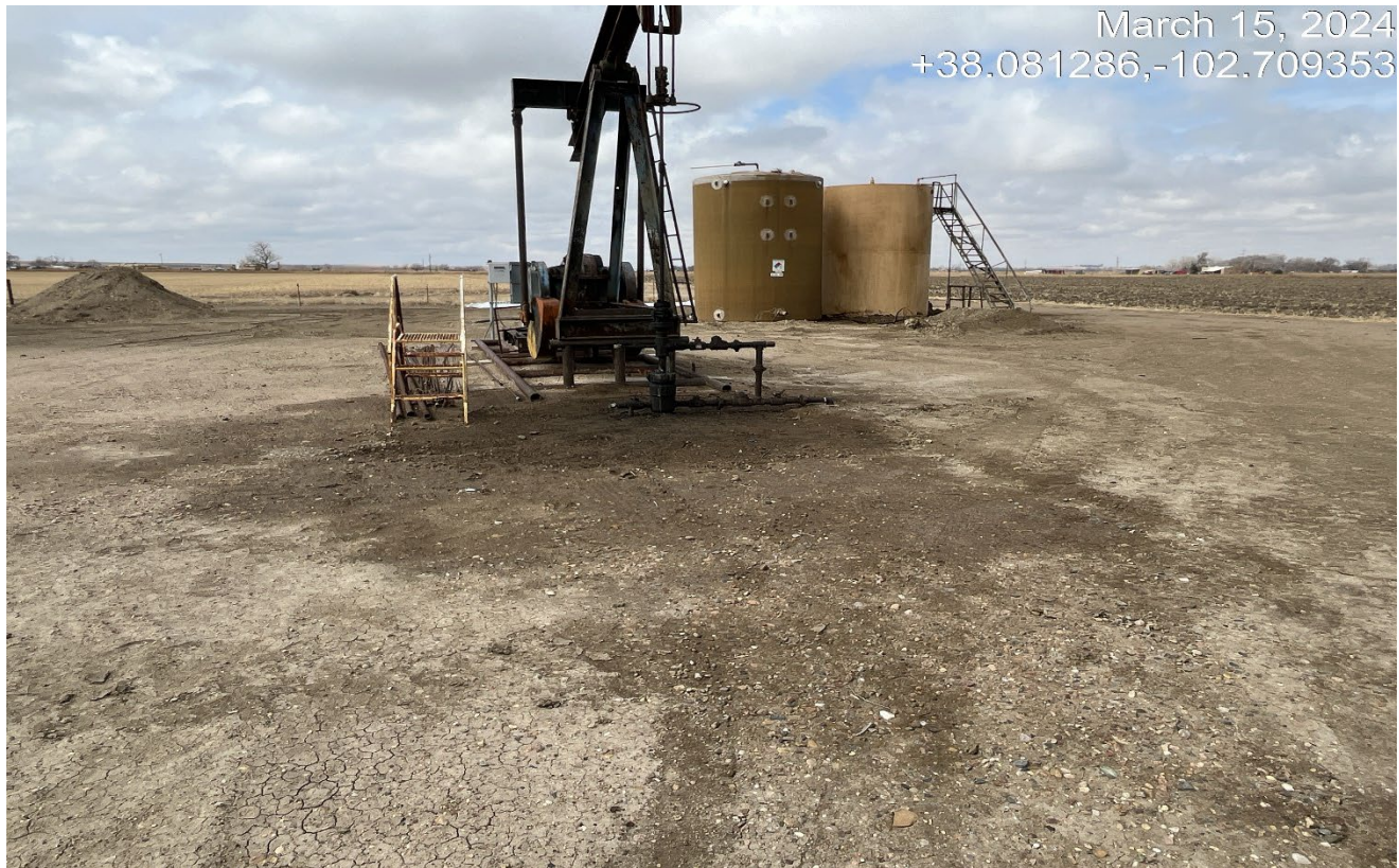
Photo 8. Facing west toward the wellhead. There is oil that has leak and sprayed out of the wellhead that needs to be cleaned up. Previous corrective action has not been completed.
