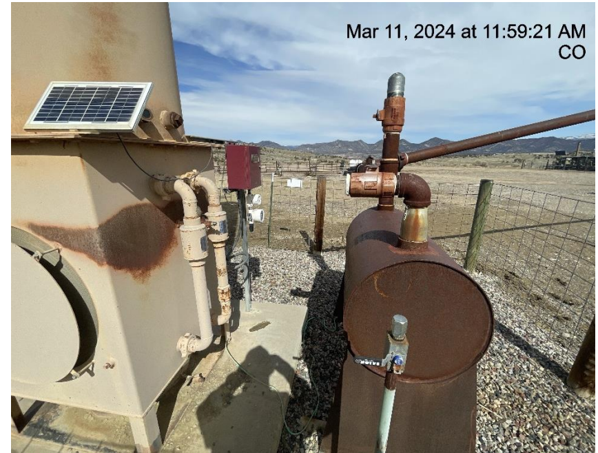
Photo # 9184 Unused equipment/ECD disconnected & not in use
