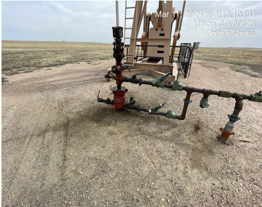
Photo 3. Photo taken facing north of staining around wellhead.
