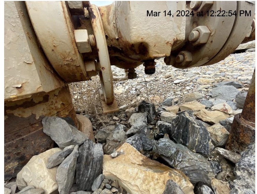
Photo # 85 Mechanical Condition - Casing valve on EF03B-19 well leaking fluid & gas
