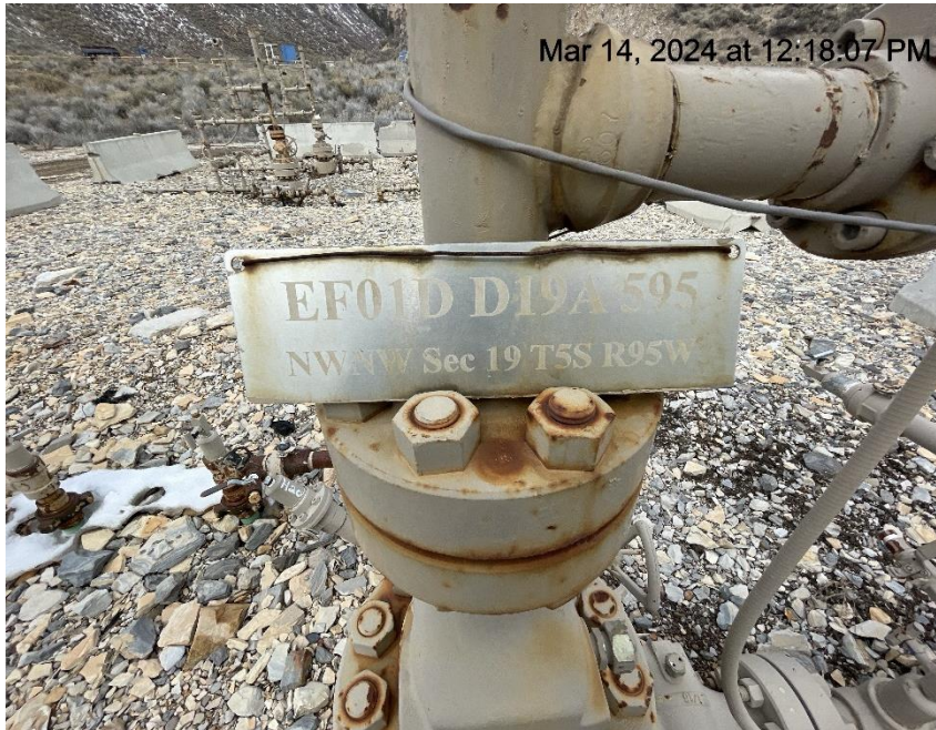
Photo # 86 Wellhead signs lack required info
